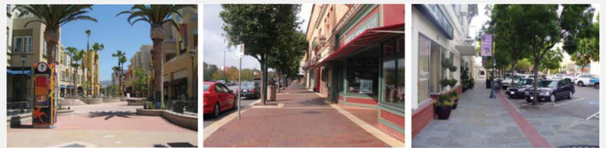
▲ Special paving across the full right-of-way ▲ Special paving in the sidewalk
